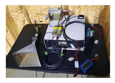
The goal was to make a +7dBm 10368 MHz signal for the antenna range source end which was battery operated and would run for at least two hours on a gel cell battery.
